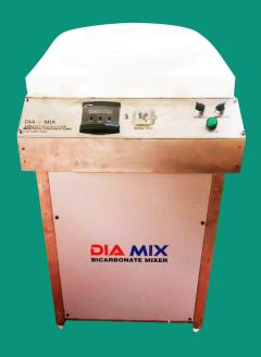
DIA MIX SERIES BI CARBONATE MIXER DESIGNED TO PREPARE A LIQUID SODIUM BICARBONATE FORMULATION FOR THE PURPOSE OF MAKING DIALYSATE FOR HAEMODIALYSIS PATIENT THERAPIES. WE USED SS 304 AGITATOR.
